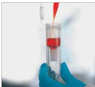
Large numbers of samples can be processed in parallel. The low hold-up volume ensures high solute recovery with minimal non-specific absorptive losses.
