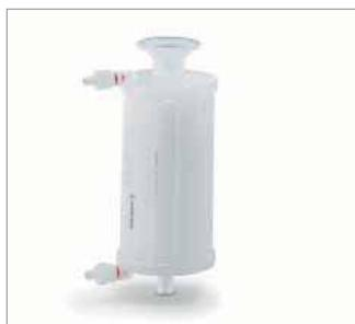
Sartobind® ion exchange capsules with 4 mm bed height are designed to remove contaminants, e. g. DNA, host cell proteins, endotoxins, leached ligands and viruses, at accelerated flow rates in flowthrough mode. This is a direct result of negligible mass transfer effects and is made possible by the > 3 µm macroporous membrane. The design allows for robust chromatographic separations and drastically reduced validation costs.
