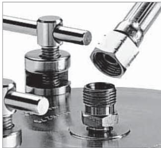
The nuts also fit on a function piece with quick-connect coupling (Order no. 6985128) for quick and simple connection to holders fitted with quick connect nipples. The valve in the coupling opens when it is fitted on a quick connect nipple, and closes when removed from the nipple.
