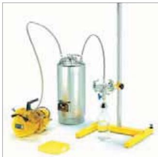
This holder is very often used in laboratories for particle removal and for sterile filtration of several liters of volume. It has a stable construction and is easy to operate. The large filtration area of 130 cm<sup>2</sup> ensures high flow rate for the total filter volume. The supplied unscrewable hose nipples can be replaced by G<sup>3</sup>/<sub>8</sub> connectors, if systems with particularly practical handling is required.
