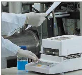
The MA35 is the basic model in the moisture analyzer series from Sartorius. Its performance functions and operating concept are geared toward daily routine processes such as repetitive QC monitoring of samples as performed during in-process control and incoming goods inspection. To make the MA35 even more user-friendly, we have done away with seldom-used programming options without compromising flexibility or measurement accuracy.
