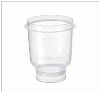
The funnel is made of polypropylene and thus is elastic enough for optimal sealing with a Click-Fit closure. Graduations are marked to allow accurate sample volumes. The large inner diameter ensures a high flow rate. The optimized shape allows thorough rinsing of the system subsequent to filtration. No liquid is retained in the filter funnel.
