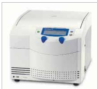
The centrifuge 2-16PK and all larger models have an automatic rotor recognition to prevent overspeeding. In addition, these centrifuges can calculate g-forces from rpm values and vice versa. As an option, free programming makes it possible to define and store individual centrifuge runs.
