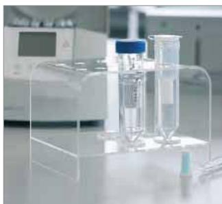
The Vivapure® mini|maxiprep MC kit is designed for simple, rapid His-tagged recombinant protein purification from a cell lysate under native or denaturing conditions. Vivapure® spin columns replace lengthy and expensive chromatographic methods such as FPLC®. Metal chelate affinity chromatography is a rapid onestep purification, which removes most contaminants and can achieve purities close to homogeneity.
