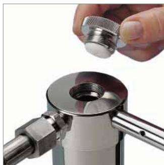
A practical holder for many laboratory filtrations. It can be attached to a tripod with the help of a steel rod which can be screwed in. The hose nipple is screwed into the side of the top part, leaving room for a large filling opening. This makes pouring in the sample easier, and the sample can be refilled without removing the tube connection to the pressure source. Leak-proof sealing is achieved by hand-tightening the closing ring.
