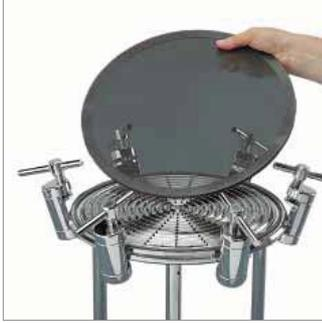
The construction of this holder is the same as that of the 142 mm holder described on page 93, except for the legs and the number of locking clamps. The three legs are made of stainless steel in order to avoid corrosion problems, as is sometimes the case with aluminium legs. They are shorter and screwed in vertically to give a very stable footing to the holder with a larger diameter. The swing-out mechanism of the locking clamps is very practical, as there are 6 clamps.
