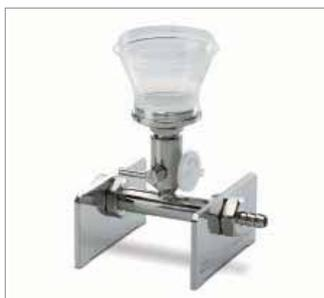
A Sartorius Stedim Biotech 47 mm gridded membrane is placed on a stainless steel filter support. A Microsart® Funnel is simply and practically fitted on. The sample is filtered.
