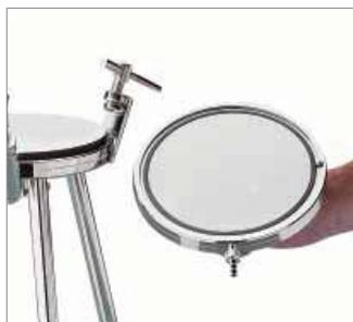
The major use of all three glass fiber filters is as a depth prefilter, placed directly on top of a membrane filter, whereby the prefilter diameter specified for the holder must be used. Larger diameters would intrude under the sealing ring of the holder and cause leakage.
