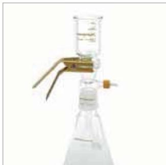
All areas, where liquid and device can come into direct contact, are made of glass or PTFE. The device, in combination with solvent-resistant, hydrophilic RC-membranes (Type 184, see page 22), is therefore ideal for ultracleaning and degassing solvents and solvent mixtures for HPLC, GC and AA.
