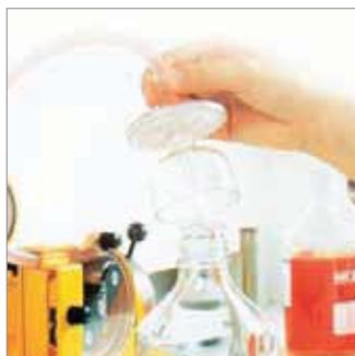
Ready-to-use units which, attached to a membrane pump or tube pump, quickly and reliably sterilize 100 ml to 5 liter of media and aqueous solutions.
